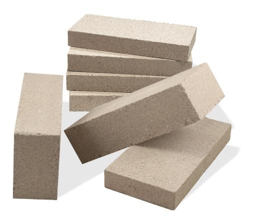
Mutual Materials Firebrick is manufactured to comply with the physical properties and characteristics specified by ASTM C 1261, Standard Specification for Firebox Brick for Residential Fireplaces. They are specifically designed for use in wood inserts or stoves and are not meant for exposed outdoor use, veneer wall or horizontal paving applications.
