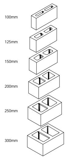
Concrete masonry units are made in various sizes and shapes to fit different construction needs. (See *Section 3.1 – Masonry Standards Commentary* for additional information) Typical shapes include stretcher; double end; half unit; bond beam; half-high unit; H-block unit; multi block unit (See over). Each size and shape is also available in various profiles and surface treatments.
